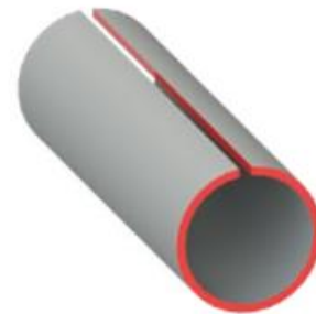
No crowning deformation
