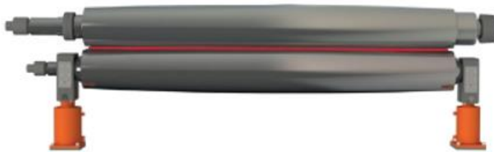
Bending thickness is compatible with roll crowning
