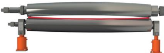
Bending thickness is thicker than roll crowning
