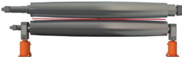
Bending thickness is thinner than roll crowning
